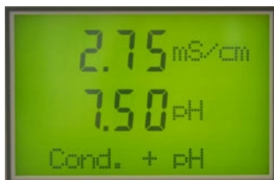
Simultaneous Conductivity and pH Measurement
